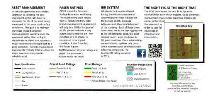
**Pavement Surface Evaluation and Rating (PASER)** is a tool to rate the current surface condition of roads.
